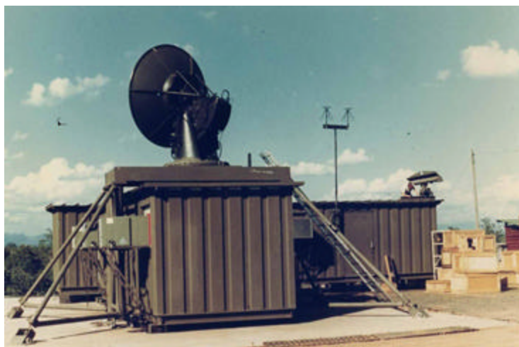
Transportable TSQ-81 systems (above) provided radar tracking coverage over the Hanoi area. This allowed B-52s to accurately strike targets and minimize collateral damage by flying to specific
